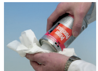
Pre-treatment of the backside / bonding side with Easy Clean Wipes
